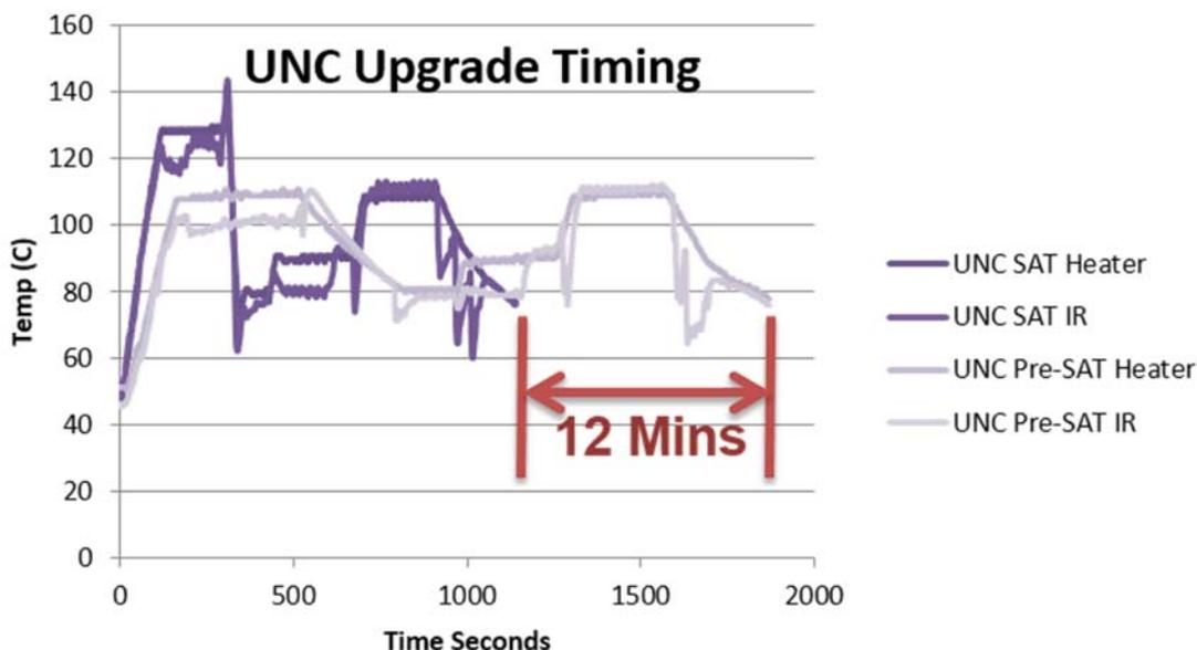
**Figure 7.** Plot comparing the 30 minute heater and infrared (IR) profiles between the current (light purple) and 30 minute cycle time (dark purple).
