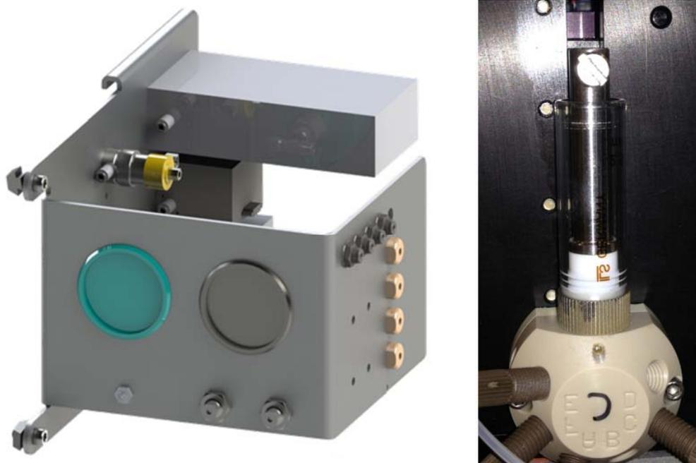
**Figure 5.** (Left) The gas manifold was updated with active cooling components. (Right) Syringe size was increased from 250µL & 500µL syringes to 1.0mL & 2.5mL. This reduces the number of strokes and therefore reduces the time for each injection. All syringes now larger than their highest respective process requirement. Air chase can be metered with reagent to reduce inject strokes.
