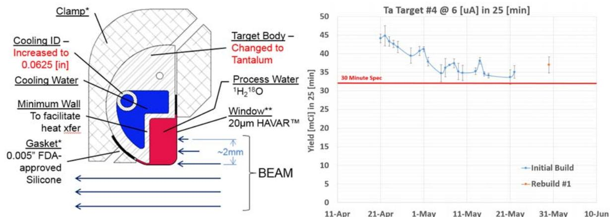
**Figure 2.** (Left) Schematic top view of Tantalum Target. The increased diameter cooling inlet line and Tantalum target body are shown identified. (Right) Tantalum Target #4 Yield.
