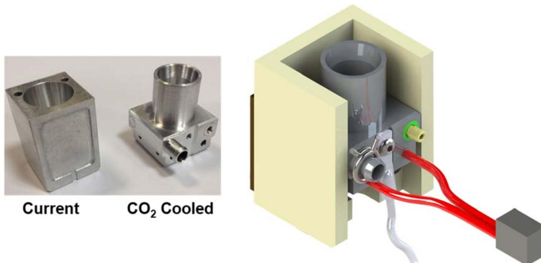
**Figure 3.** Active cooling block used to cool the temperature of the reaction chamber. It has a lower mass, an internal chamber for CO<sub>2</sub> cooling and results in improved heater mounting.
