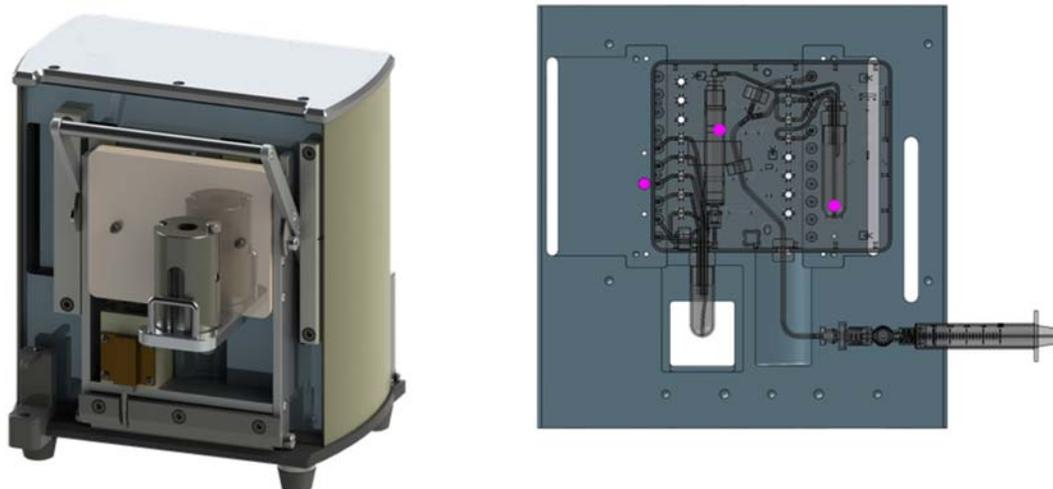
**Figure 4.** The Chemistry Card System (CCS) faceplate requires update to accommodate the active cooling and bulkhead fittings for CO<sub>2</sub> cooling.
